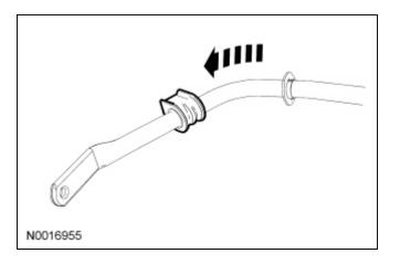
3. **NOTE:** To aid installation, apply a light coat of lubricant to the necessary parts of the front stabilizer bar and the inside diameter of the stabilizer bar bushing.
